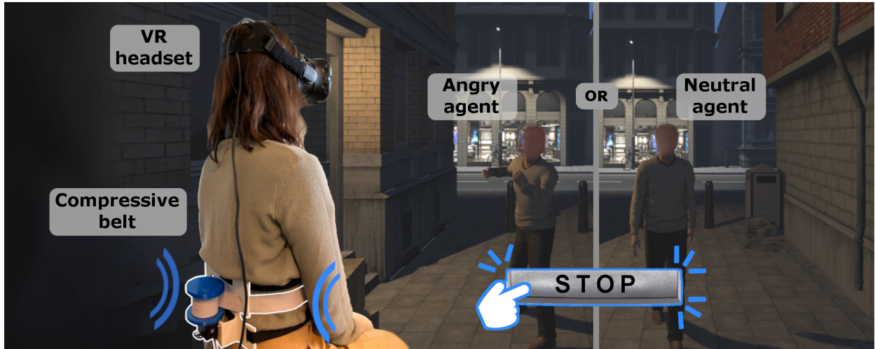
Fig. 1. Users immersed in a virtual dark alley watch a virtual agent slowly approaching them. The teaser image was lightened to enhance visibility. The agent can visibly emote anger or appear neutral, and as he advances, a belt wraps around the users' torso, simulating the users' shrinking peripersonal space. When feeling uncomfortable or threatened, users can choose to stop the progression of the agent by pressing a button. Results show that the body language of the agent and haptic stimulation of the observer both significantly influence users' perception of threat and their peripersonal space.
