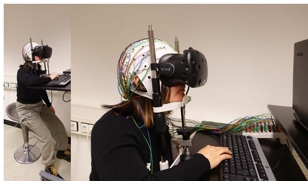
Fig. 2. VR-chin rest-EEG setup shows a participant standing against the height-adjustable bar chair.
